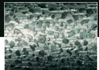
The surface of a STROH ROLLER DRESSER covered by infiltrated and statistically distributed diamond grain (IS type).
