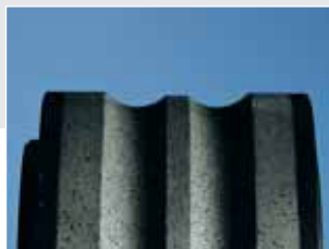
STOH ROLLER DRESSER for grinding the raceway of a ball bearing.
